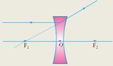
(ii) A ray of light appearing to meet at the principal focus of a concave lens will emerge parallel to principal axis.
