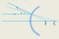
(iii) A ray directed towards the center of curvature of a convex mirror is reflected back along the same.
