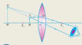
Position – On the same side of the lens as object Nature – Virtual and erect Size – Enlarged
